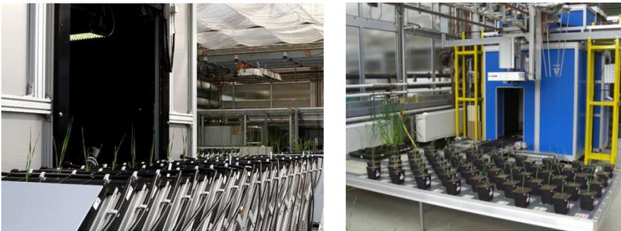
Fig. 1: The GROWSCREEN-Rhizo prototype system (left) and the Automated Shoot Phenotyping Platform (right) allow the quantitative measurement of total shoot projected area and of the visible part of the root system
