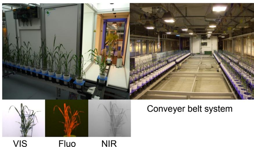
Fig. 1: The LemnaTec-Scanalyzer 3D system in IPK. Left side: imaging chambers for visible, fluorescence and near-infrared wavelengths; Right side: conveyer belt system
