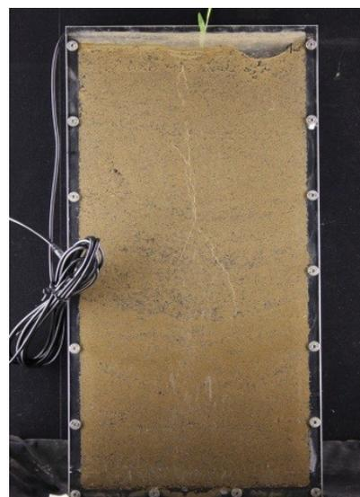
Fig. 3: Three weeks old barley plant growing in a rhizotron (60cm x 30cm x 3cm). The volumetric water content was monitored by Frequency Domain Reflectance sensors
